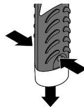
1. Press the pressure areas on both sides and pull the battery compartment cover off the device.
