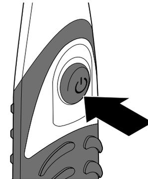
3. To turn the device on **briefly**, press the On/Off switch. The brush will rotate for as long as you keep the On/Off switch pressed.
